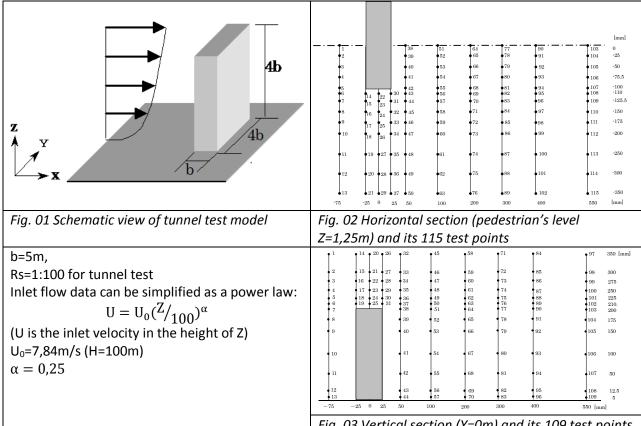
Fig. 03 Vertical section (Y=0m) and its 109 test points
