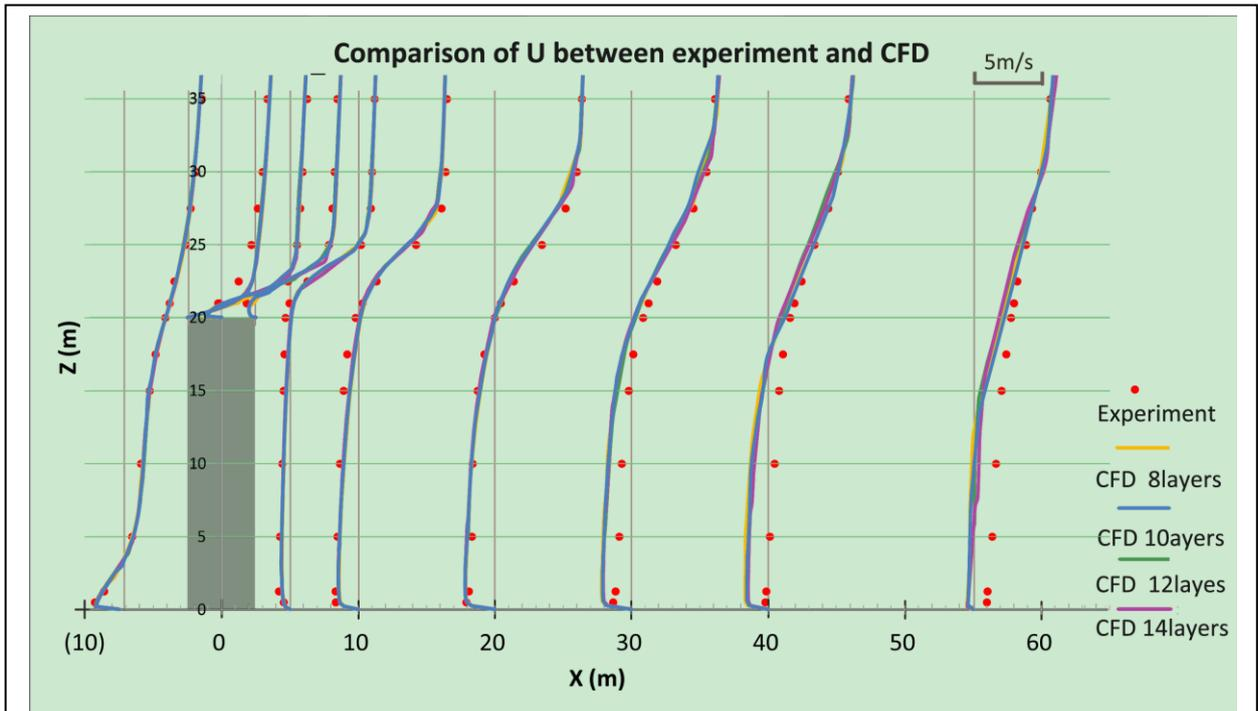
Fig. 06 Comparison of results CFD with meshes of different inflation layer numbers (N)
