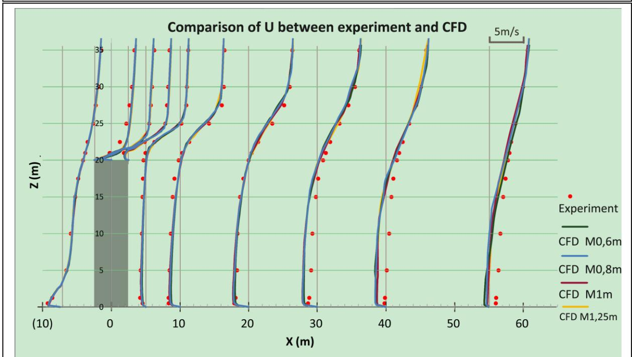
Fig. 07 Comparison of results CFD with meshes of different size precision for the building (N)
