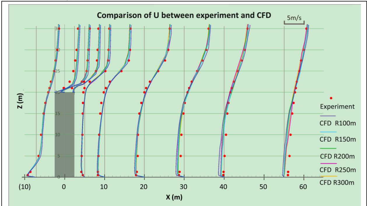
Fig. 04 Comparison of results CFD with model in different domain scales
