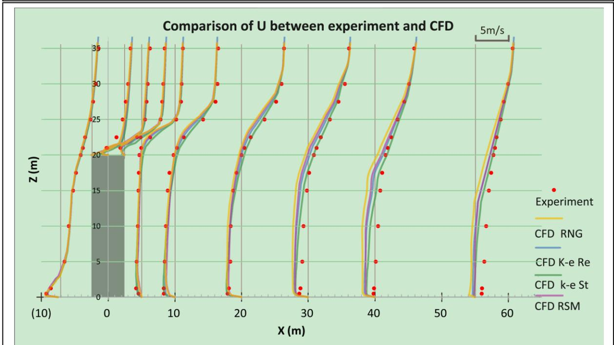
Fig. 05 Comparison of results CFD with different turbulent models
